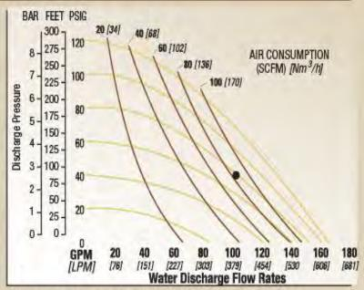
Flow rates indicated on chart were determined by pumping water.
