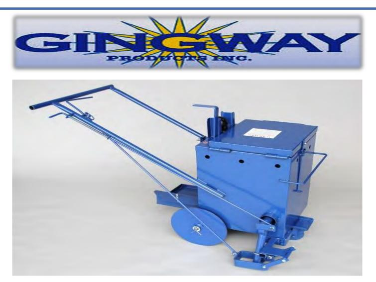
MA10 Melter/Applicator is a fast and efficient method for the application of hot applied crack sealants. It can also apply materials from stationary kettles or any large Melter. It can be used without heat for cold pour materials. It is capable of melting and applying 600 lbs. of sealant per day.
